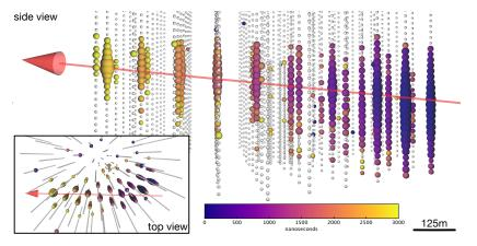
Neutrino produced high energy muon near IceCube. Muon produced light as it traverses IceCube volume. Light is detected by array of phototubes of IceCube.
